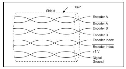
Figure 15. Shielded Twisted Pairs
